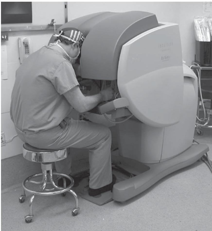
Fig. 4. The da Vinci surgeon's console, from which the robotic camera and instrument arms are controlled.
