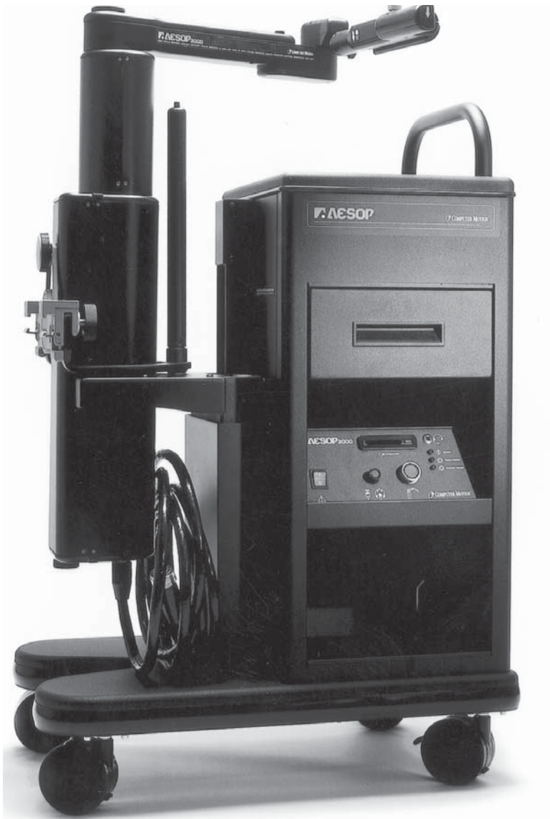
Fig. 1. The Aesop robotic arm. It can be mounted to the operating table and accommodates most conventional endoscopes.
