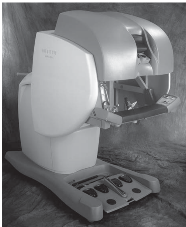
Fig. 1. Da Vinci surgical telemanipulation system: surgeon's console.
