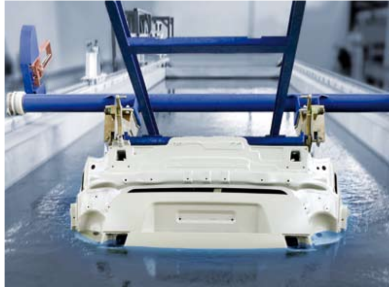
Integrated RoDip conveyor technology for a high level of corrosion protection
